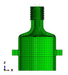
131059 Nodes 61368 Elements (C3D20, C3D10) Local coordinate systems (elementwise definition)
