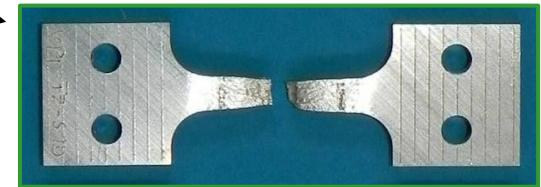
Plastic straining and fracture can be strongly orientation dependent
