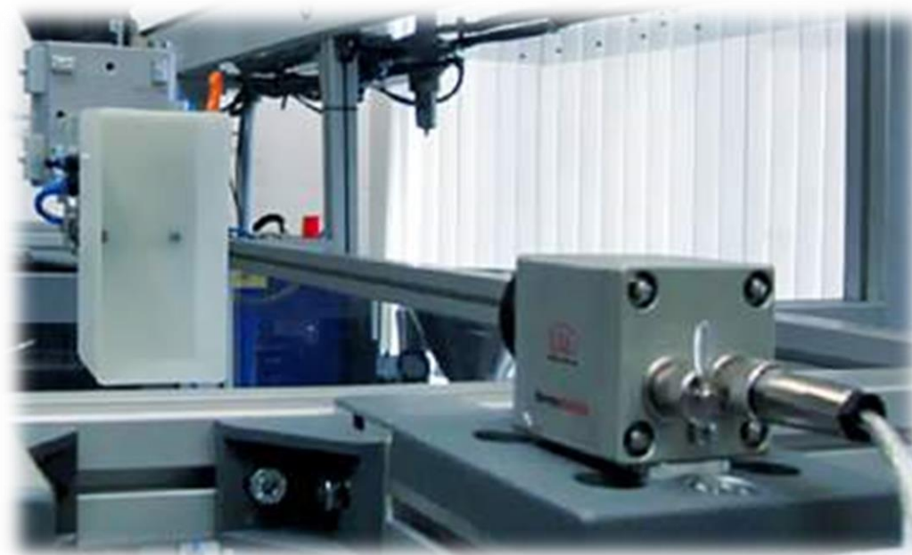
Experimental Setup: Ejection Temperature measured by IR
