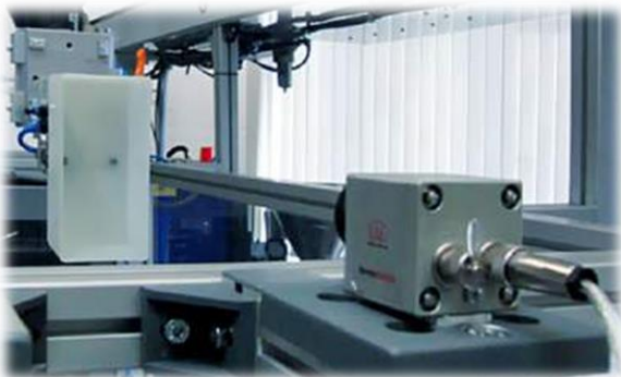
Experimental Setup: Ejection Temperature measured by IR
