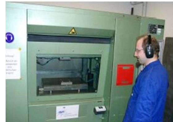
Vibration Welding Machine (Branson)
